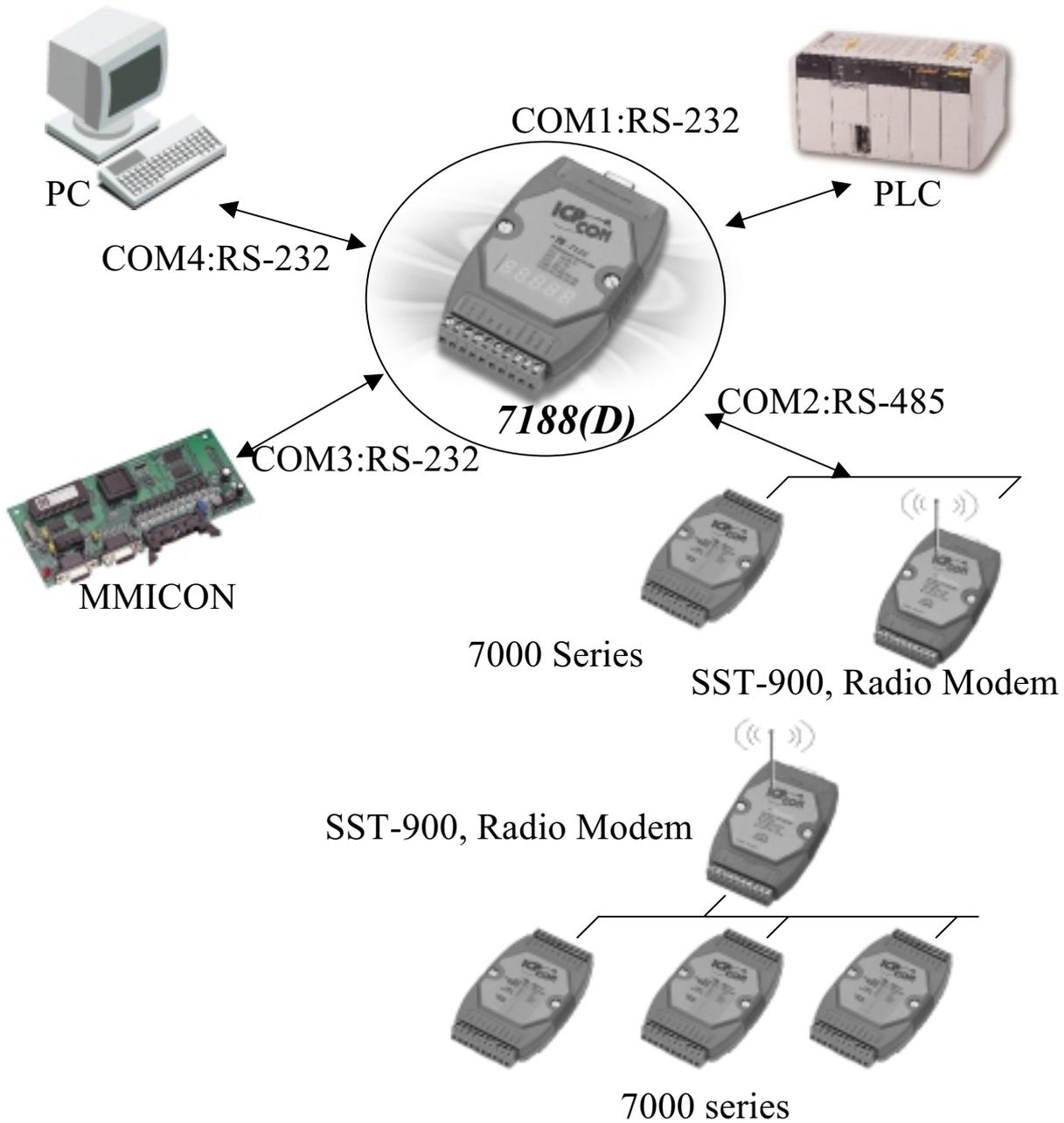
COM1: PLC can access the I/O states of 7000 modules
