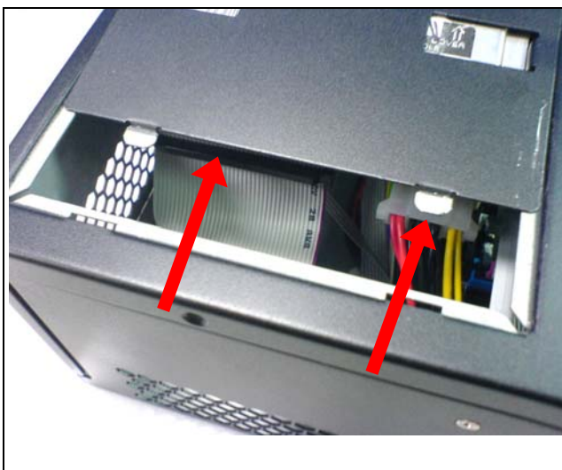
Fig. 5-5 Connect IDE cable and power connector to 3.5" HDD
