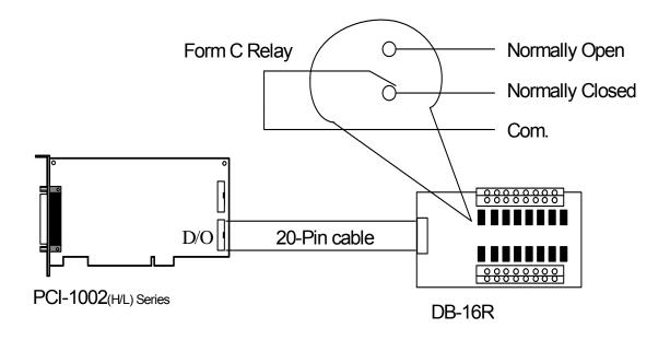
PNote: Channel: 16 Form C Relay Relay: Switching up to 0.5 A at 110 Vac or 1 A at 24 Voc
