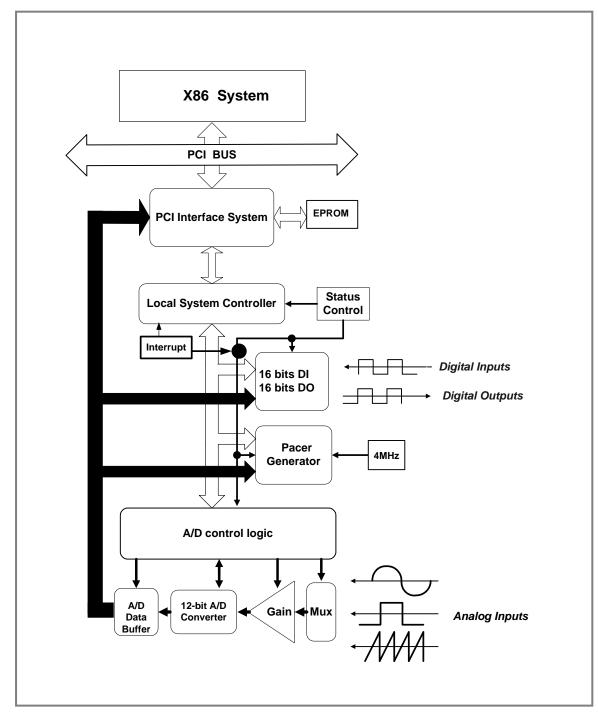
Figure 1-1: The PCI-1002 series block diagram.
