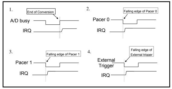
Figure 1-3: Programmable interrupt source.
