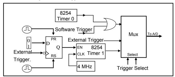
Figure 5-3: A/D trigger controller.
