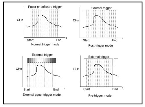
Figure 1-2: Trigger methods of PCI-1002 series.
