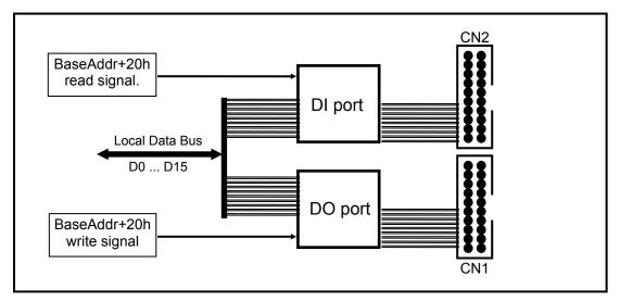
Figure 5.1: DIO function diagram.
