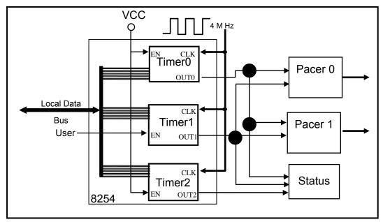
Figure 5-2: 8254 control diagram.
