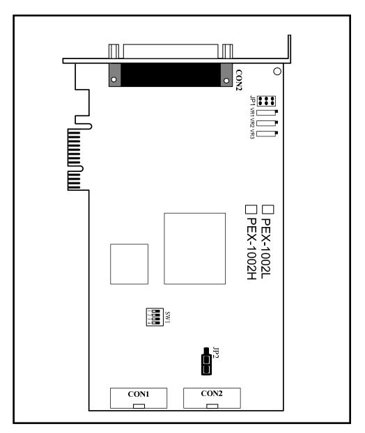
Figure 2-2: PEX-1002 board layout.
