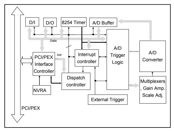
Figure 2-2: PCI-1002 series System Function Block.
