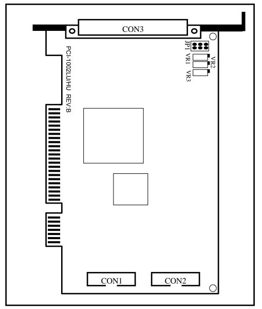
Figure 2-1: PCI-1002 board layout.
