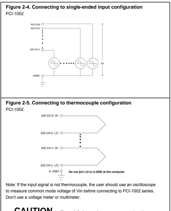
**CAUTION:** In Figure 2-5, the maximum common mode voltage between the analog input source and the AGND is 70 V<sub>p-p</sub>. Make sure that the input signal is under specification first! If the common mode voltage is over 70 V<sub>p-p</sub>, the input multiplexer will be permanently damaged.
