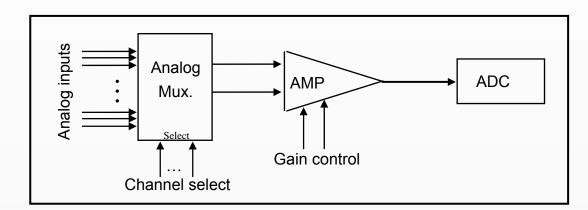
Figure 4-2: Analog input control.
