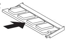
Push the DIMM gently downwards until the slot levers click and lock the DIMM in place.
