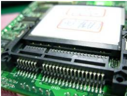
Installing the CFAST in the back of the board. Note that the slot direction and fool-proofing
