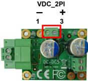
VDC\_2PI: Terminal Block 2-pin power connector
