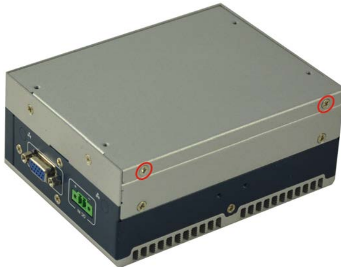
Figure 3-14: Reinstall the Bottom Panel (ITG-100-AL-E1)
