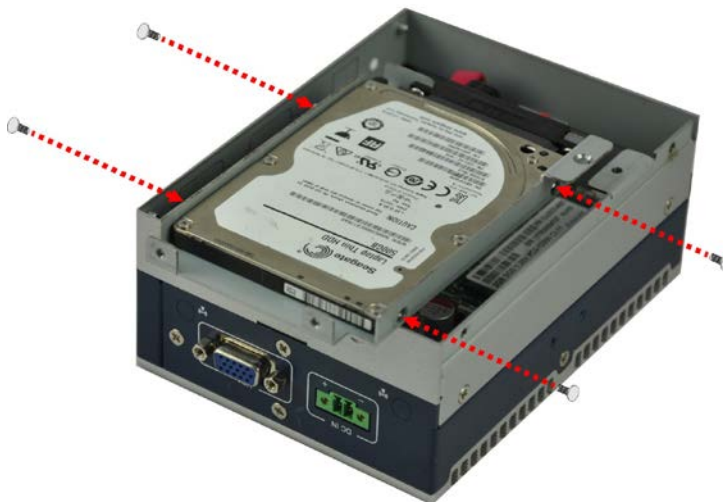
Figure 3-3: Install the HDD
