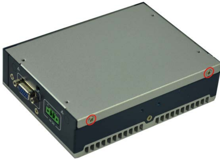
Figure 3-11: Remove the Bottom Panel (ITG-100-AL-E1/S)
