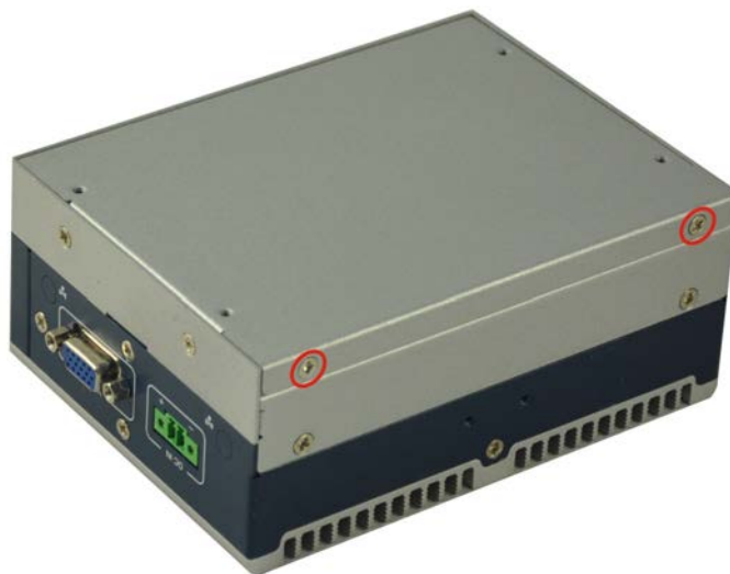
Figure 3-1: Remove the Bottom Panel
