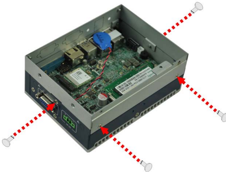
Figure 3-12: Additional Block Layer Installation
