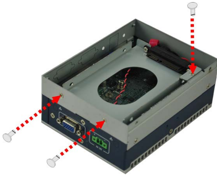
Figure 3-13: HDD Bracket Installation
