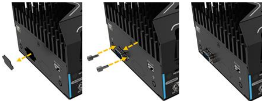
Figure 3-17: Knock out the reserved holes
