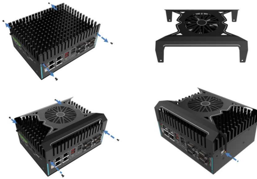
Figure 3-19: External Fan Module Installation
