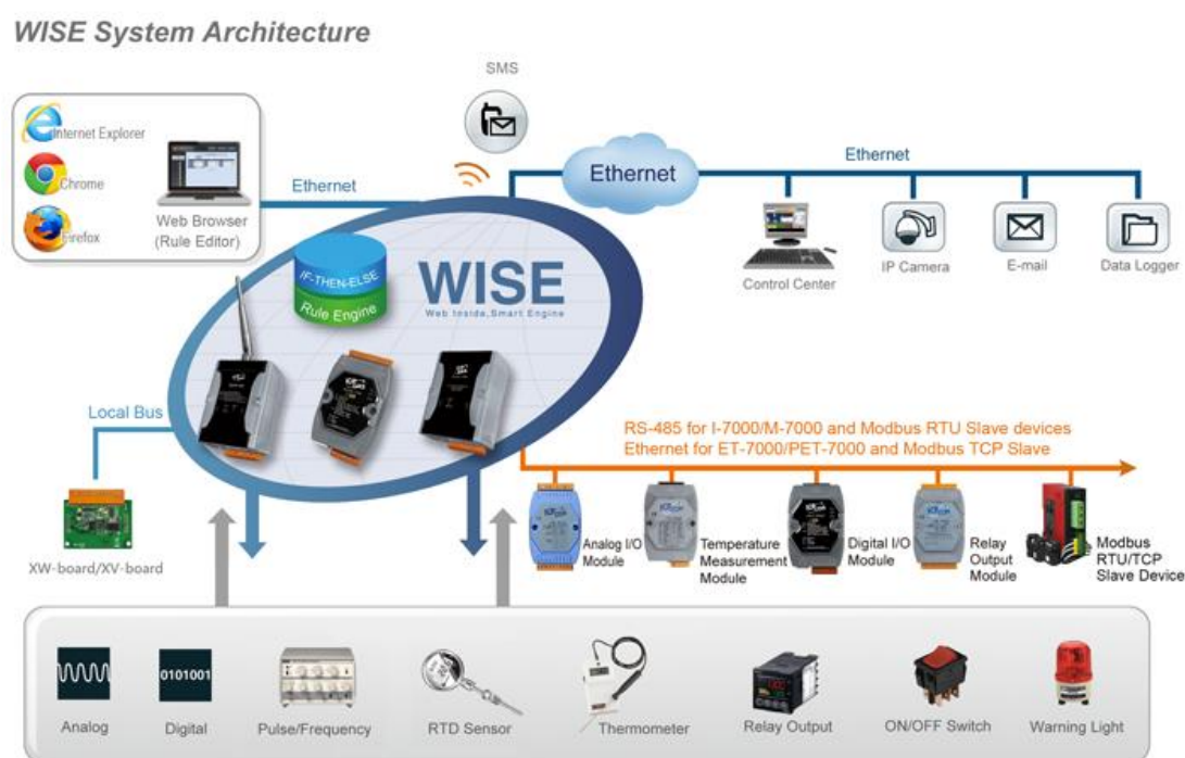
Figure 1-1 : WISE system architecture
